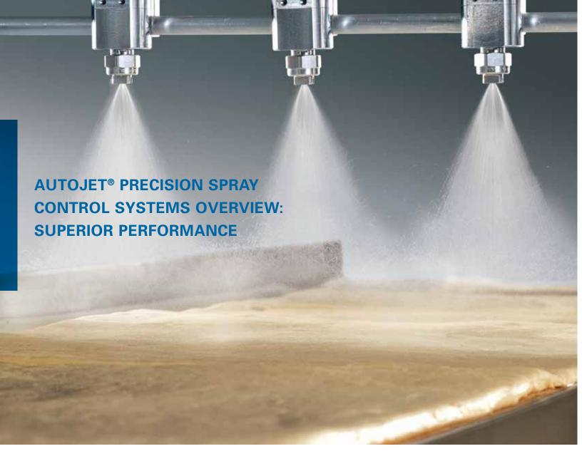
AutoJet® Precision Spray Control Systems consist of PulsaJet® automatic spray nozzles and an AutoJet spray controller. Many systems also include a spray manifold. These systems use Precision Spray Control (PSC) to ensure coatings are applied consistently, uniformly and with minimal waste even when conveyor line speed changes.
